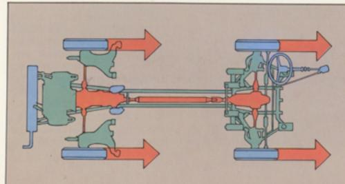
differential begins to transfer power to the front wheels. This permanent four wheel drive system engages smoothly and automatically whenever it senses gallon fuel tank. a difference in speed between the front and rear axles. The result is dramatically improved traction and directional control.
