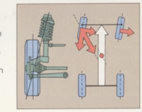
The Volkswagen Vanagon's semi-trailing arm rear suspension features independently mounted coil springs and doubleaction shock absorbers to provide accurate guidance of the rear wheels for better tracking and long tire life.
