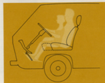
Steering wheel angle, pedal height and seating were ergonomically designed to suit about 95% of the population.
