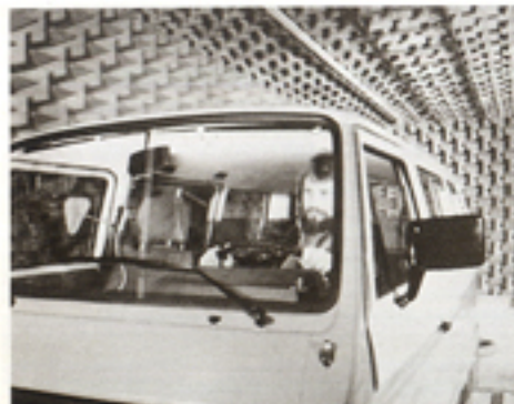
Sound-deadening insulation was put to the test in an acoustical chamber.
