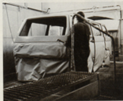
A worker masks the body prior to application of a second color.
