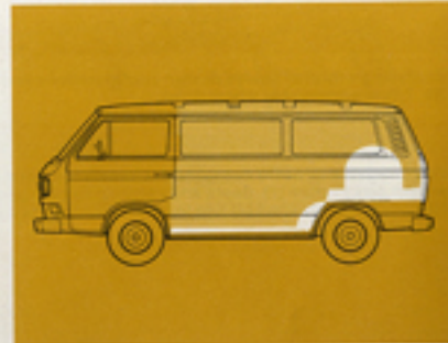
Lowering floor and engine compartment increasing interior capacity by 40%.
