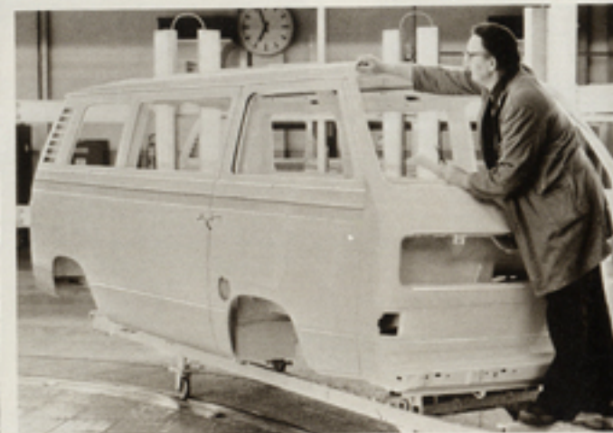
A paint inspector checks the finish.
