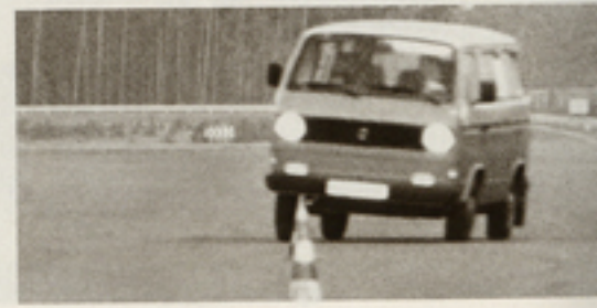
Proven at Ehra-Lessien: Wider track, longer wheelbase and a well positioned center of gravity combine to give Vanagon cornering characteristics akin to some sedans.
