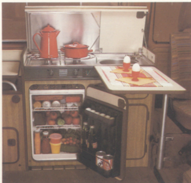
L model has 3-way refrigerator, 2-burner cookstove.
