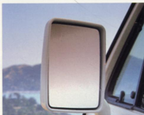
◀ For improved rear visibility and greater driving safety, oversized power remote controlled outside mirrors with built-in electric defrosters are standard (optional on Vanagon).
